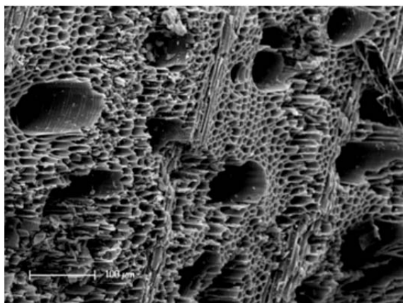
“Figure 3. Porous structure of Biochar”
